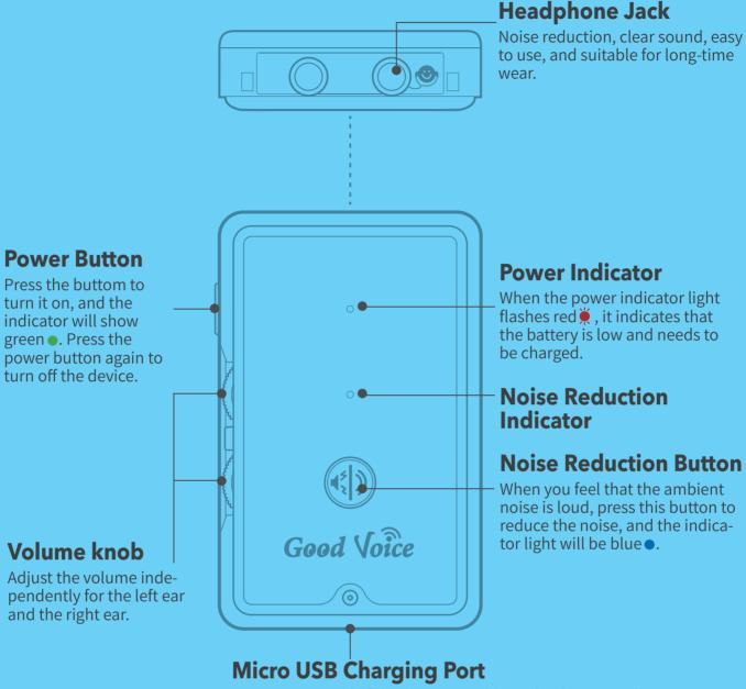
Connect one end of the charging cable to the device, and connect the charger or mobile power to the other end to charge. The power indicator light is solid red ●. When power is full, the indicator light will go out.
