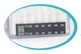
Verify Specimen Temperature(Acceptable Specimen: 90-100 ₹/32-38 ℃)
